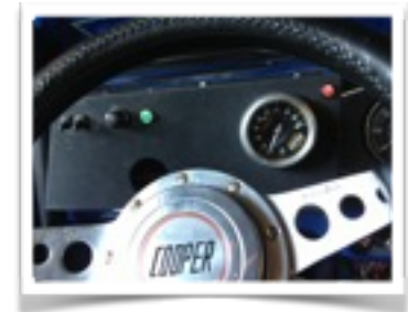
Installed and finished- wipers, washers, start button, air fuel ratio meter, speedo-
