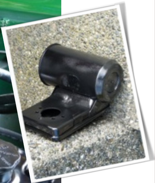
HIF intake. The mounting holes on the HIF will need to be elongated to line up with the mounting hole on
