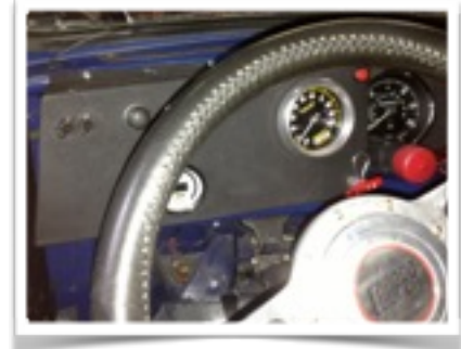
meter and horn all easily visible or accessible. The fire extinguisher cable is just visible to the lower right. The large red 'button' is an over-rev and/or overheat warning light
