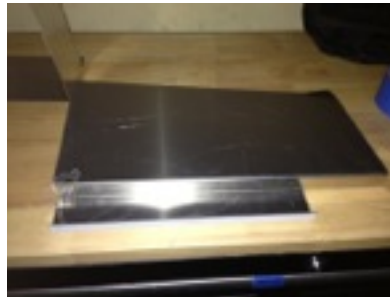
Sheet metal cut and bent to shape
