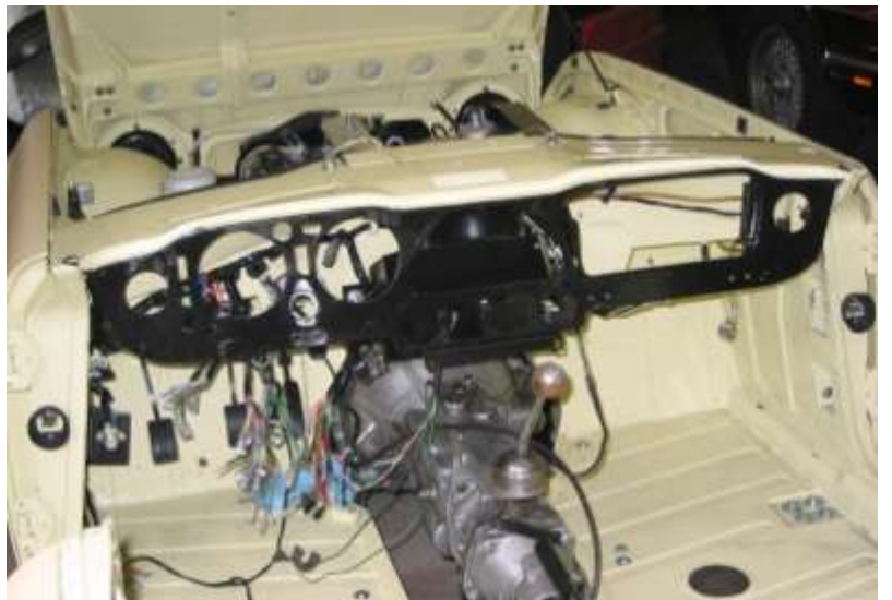
New bits going back on including the new wiring loom. Joseph Lucas would be proud.
