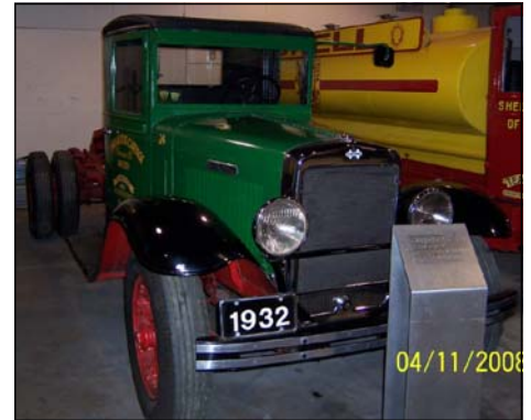
1932 International A-4 Tractor (4.88 litre 6-cyl, 98 hp): Built as a flatdeck, converted to a tractor in 1935. It was used to haul stern tubes and gun mounts to the shipyards during WWII and general freight around Vancouver until 1948.
