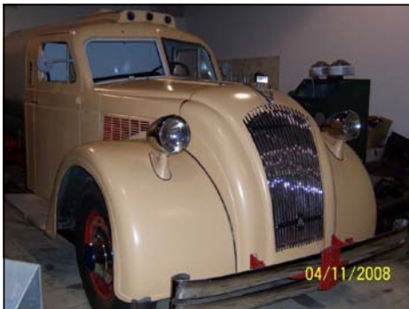
1935 Dodge K52 Airflow (5.4 litre 6-cyl, 128 hp): Standard Oil used this truck with its streamlined tank to deliver gasoline to Chevron stations in the greater Vancouver area from 1935 to 1948.
