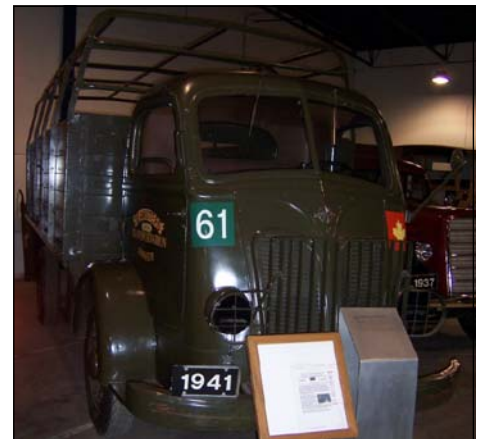
1941 International COE 2-Ton Ribtop (3.81 litre 6-cyl, 112 hp): Used by the Royal Canadian Army Service Corps, Military District 11 (British Columbia) during WWII.
