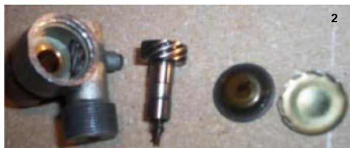
groove and I had to remove excess metal to pry loose the metal retainer.) Remove the bearing disc behind the retainer and carefully remove the worm drive pinion (into which fits the driver cable).
