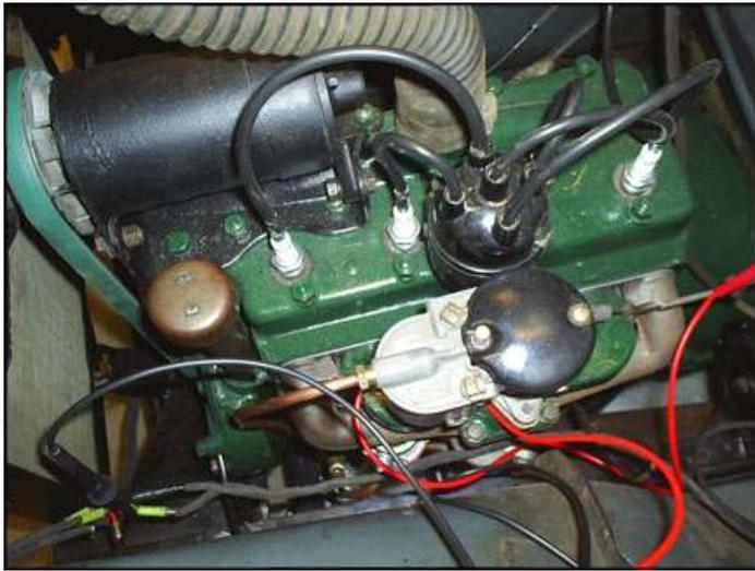
built-in oil funnel and hinged lid fitted after the war. The generator had a much different mounting. A one-piece pressed bracket sat atop the cylinder head and cradled the generator body which is of the three brush type and is mated with a simple cut-out rather than the more sophisticated regulator (and two brush generator) used later on. No oil filter was fitted nor any water pump and a small plate over the carburetor sufficed in place of an air cleaner.
